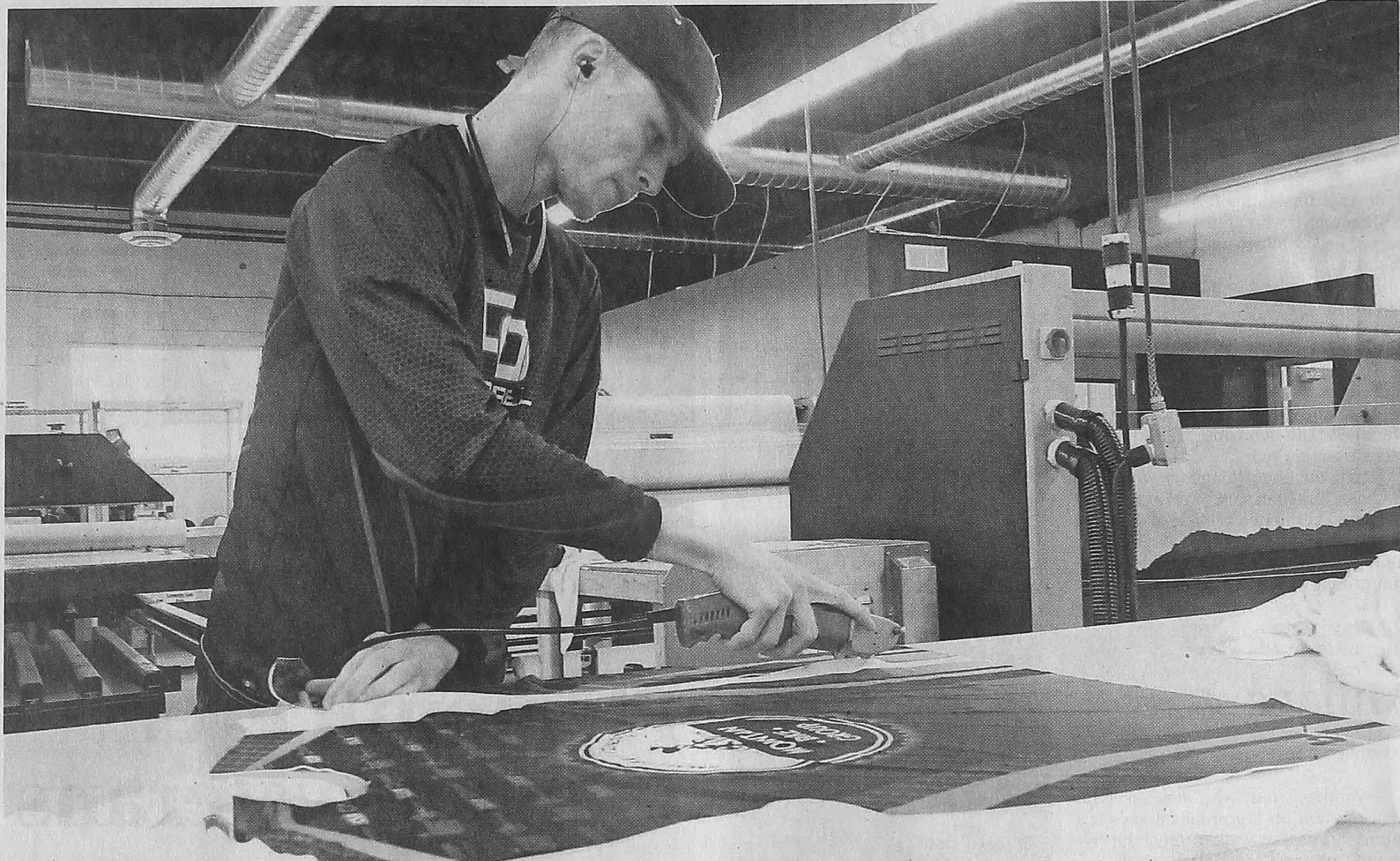
DO Apparel employee Jacob Krasinski uses an electric cutting tool to trim away excess material from jerseys before they're stitched together Oct. 29. PHOTOS BY JOHN HEIDER/HOMETOWNLIFE.COM
