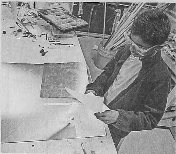
Ashwath Kumaravel cuts paper templates used for guidance when cutting sheet metal.
