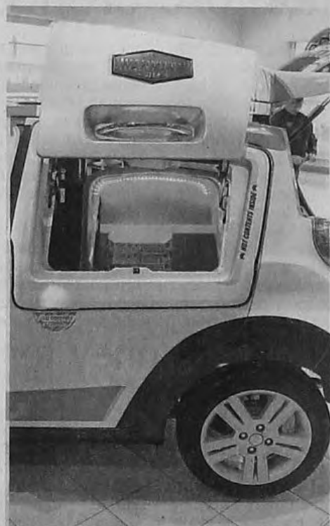
The back of the modified Spark has a chamber that keeps pizza hot for delivery.
