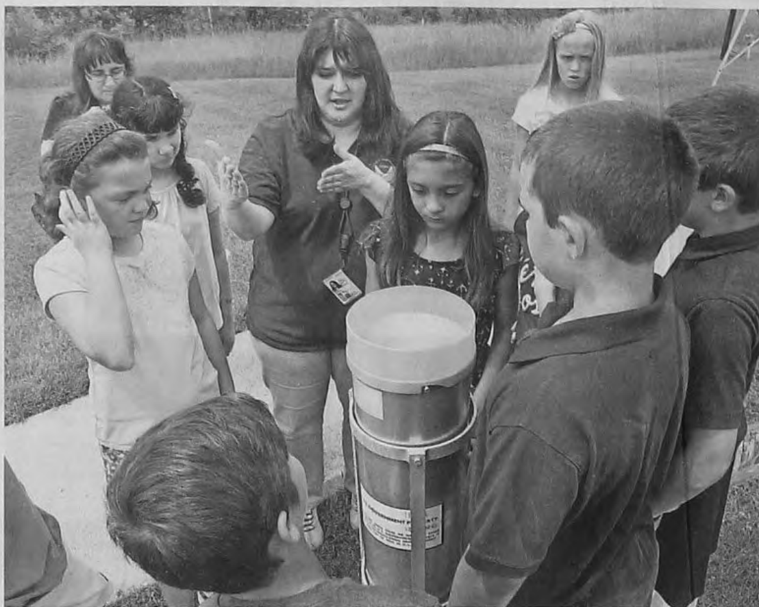
Meteorologist Heather Orow explains to students how a rain gauge operates.
