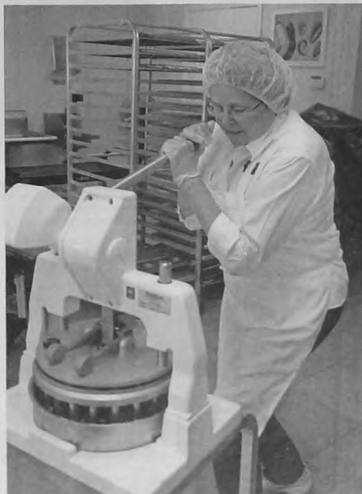
Using a machine sure beats scooping dough by hand. Julie Tenbusch presses the lever on a dough-cutting machine
