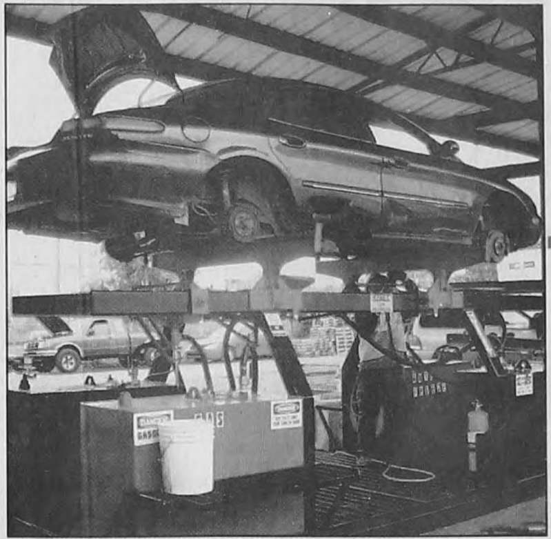
An end-of-life vehicle is carefully taken apart, piece by piece. All fluids are carefully drained and properly disposed of.
