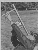
Jim Shirmer, an automotive tech teacher, uses a student-made inclinometer to measure the angle of the rocket flight, which tells the maximum height of the flight.
