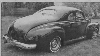
The 1941 Ford business coupe spent years upside down in a swamp in South Dakota. Bob Hayes had the vision and resurrected the car, chopping the top 5 1/2 inches, adding grillwork from a 1950 Oldsmobile, seats from a 1980 Thunderbird and powering it with a 1951 flathead Ford V-8.
