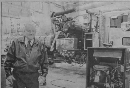
Jack Doheny, president and founder of the Northville-based Jack Doheny Companies, walks past one of his company's signature trucks: a Victor 2100 model. The truck, which run about $500,000, is used to clean up oil and hazardous material spills, and is also used by most municipalities to clear jammed sewers. PHOTOS BY JOHN HEIDER (STAFF PHOTOGRAPHER)
