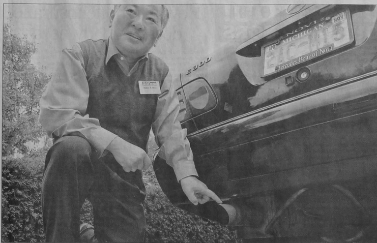
Julius Rim points to a prototype of his Green Power exhaust gas recovery system that he's installed on a diesel Mercedes. Rim, whose system helps to scrub exhaust and use part of it to heat water vapor that's then added back into the combustion process for better fuel efficiency, is hoping to get further into the automotive business. His system is already in use in maritime engines. JOHN HEDER | STAFF PHOTOGRAPHER
