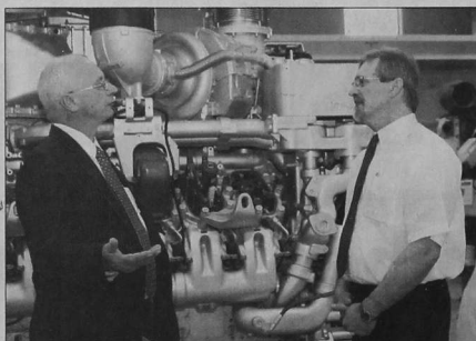
PHOTOS BY ELMA RILEY | TOGNUM AMERICA Congressman Kerry Bentivolio (left) listens as Wolfgang Griener, senior manager at the MTU Training Center in Canton, explains the MTU Series 4000 oil-gas pump engine.
