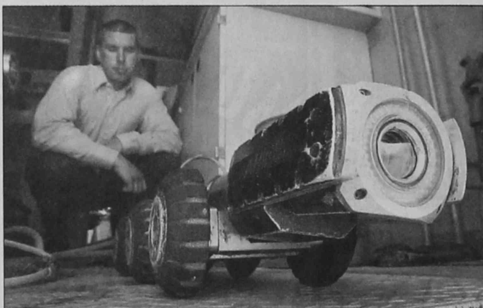
Bob Belair and the robotic camera that prowls the sewers of Canton.
