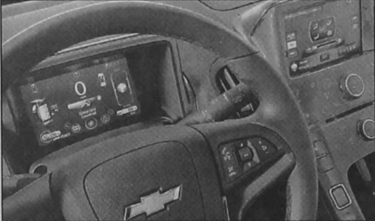
A favorite feature of Volt owners is the IP gauge that helps them closely track fuel efficiency.
