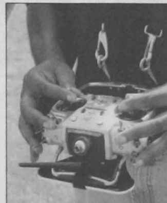
The flight controls are attached to a harness on the pilot so hands are free to operate plane.
