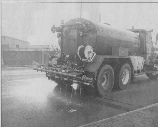
The county will begin pre-wetting roads with a salt brine solution to dissolve the salt instantly and keep it from bouncing off the roads.
