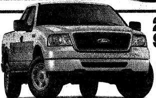
Pref Equipment Package 507A, XLT series, 5.4 L EFI V8 engine, electronic 4-speed automatic O/D transmission, P255/70RX17 OWL all-terrain tires, 3.55 ratto limited slip axle, 7150# GVWR package, electronic shift-on-the-fly, sliding rear window, keyless entry key pad, 17" mach aluminum with paint accents. Stock #62593
