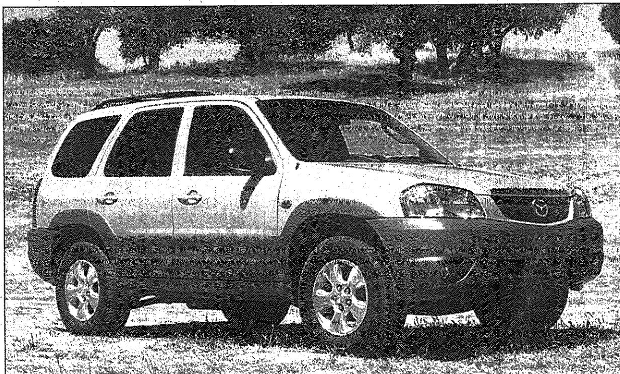
Mazda Tribute Vehicle class: Small sport utility vehicle. Power: 3.0-liter DOHC 24-valve V6. Mileage: 18 city / 24 highway. Where built: Flat Rock, Mich. Price: About $23K.
