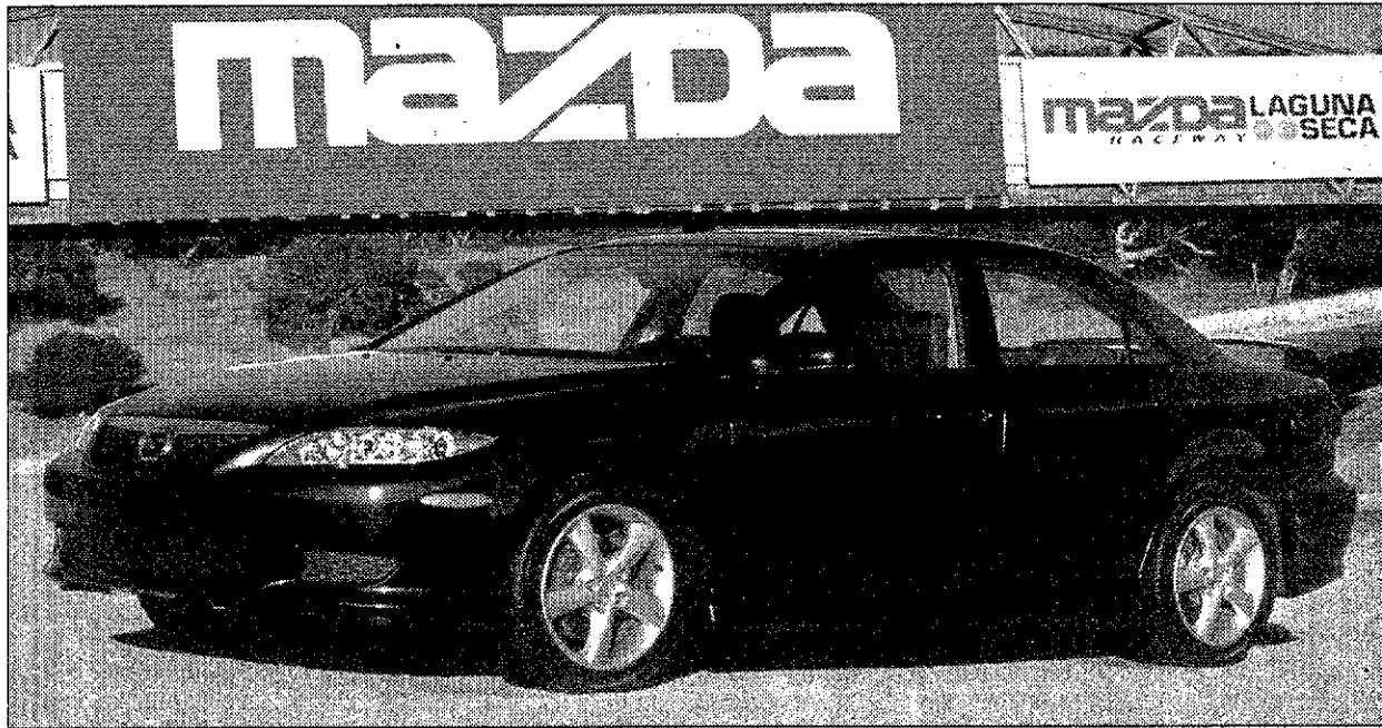
2003 Mazda 6. Vehicle type: Mid-size sport sedan. Engine: 3.0-liter dual overhead cam 24-valve V6. Mileage: 19 mpg city/27 mpg highway. Where built: Flat Rock, MI. Price as tested: $25,345.
