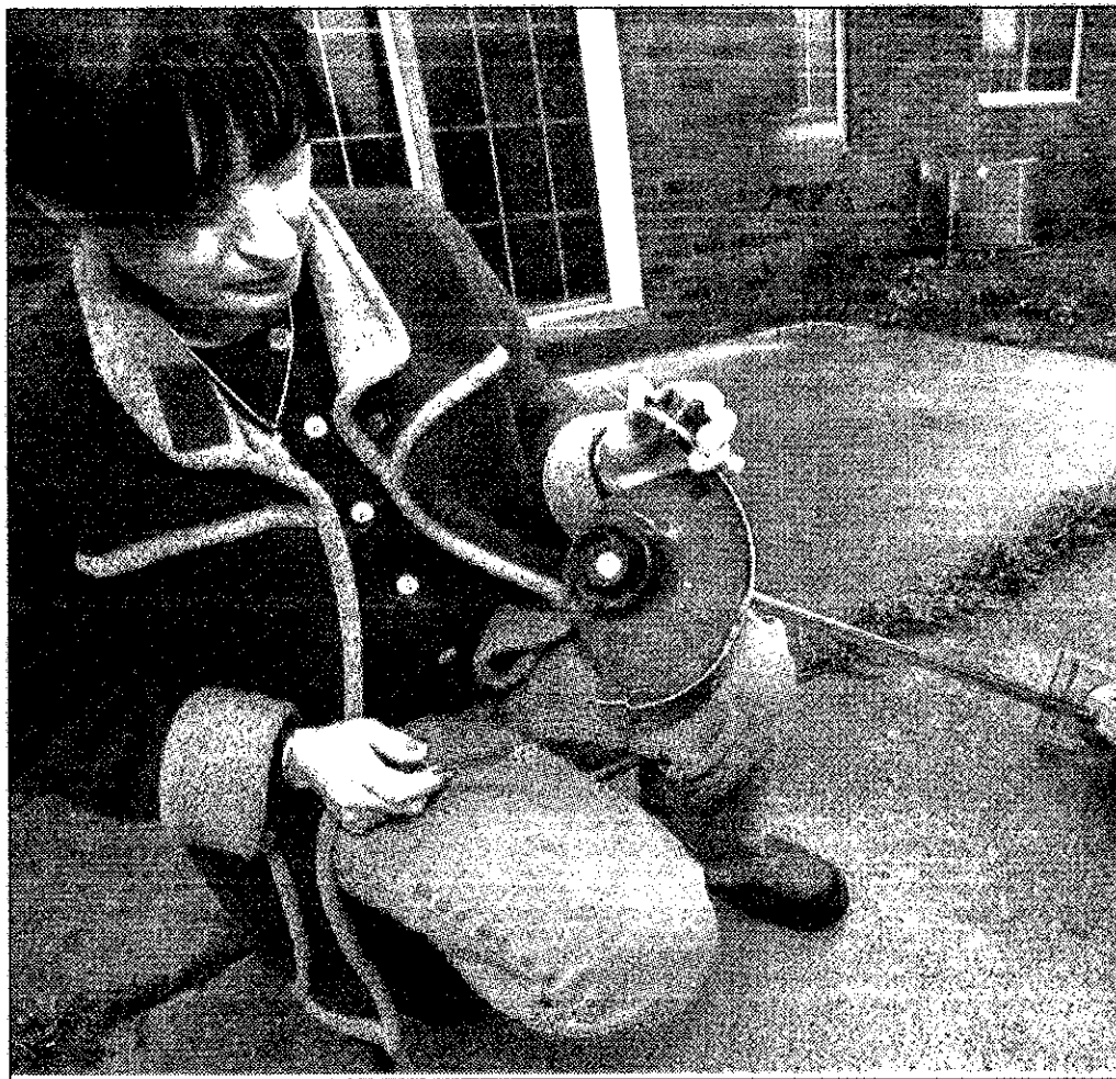
Pop the top: If your power trimmer runs out of line, just remove the cap and reline the string, using orange or yellow line, so it is easily visible. Once the line is replaced, Kluz takes the trimmer on a short test run.
