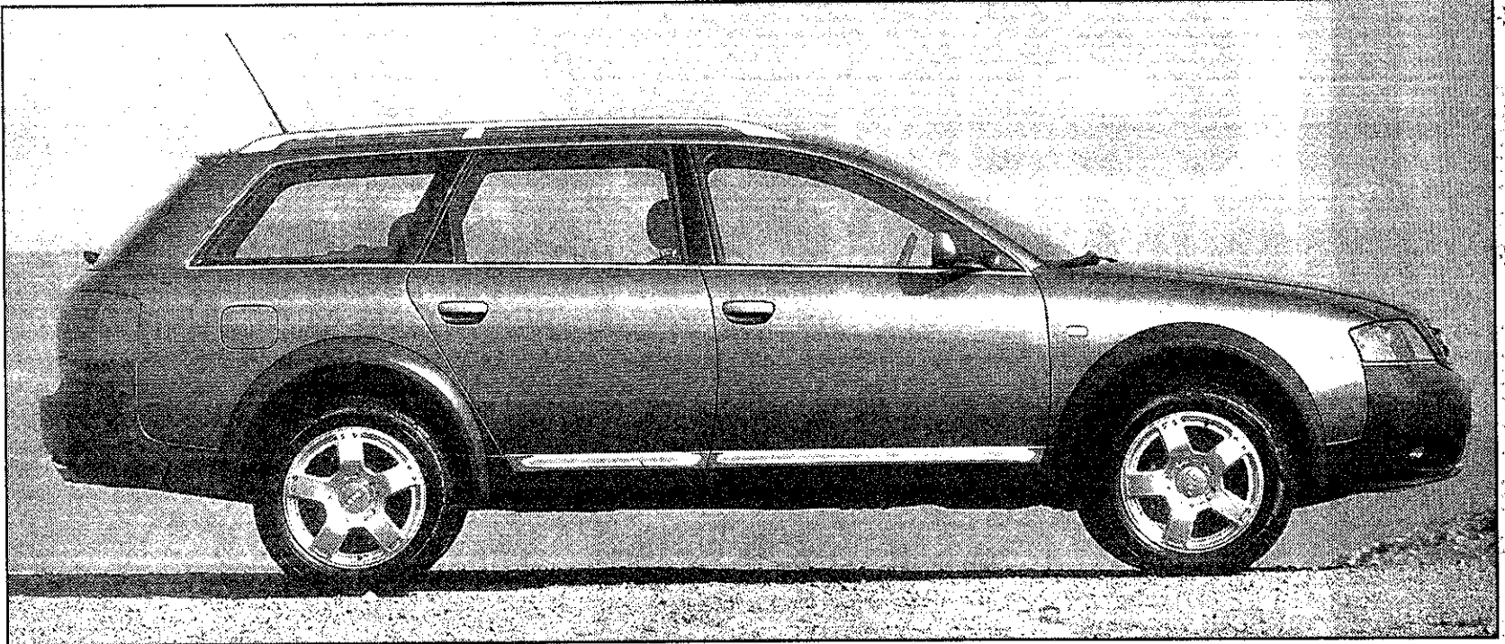
Low rider: The Audi allroad (manufacturer's lack of capitalization) is an all-wheel drive station wagon featuring a four-level, hight-adjustable pneumatic suspension that provides up to 8.2 inches of ground clearance for off-roading and 5.6 inches for highway driving.
