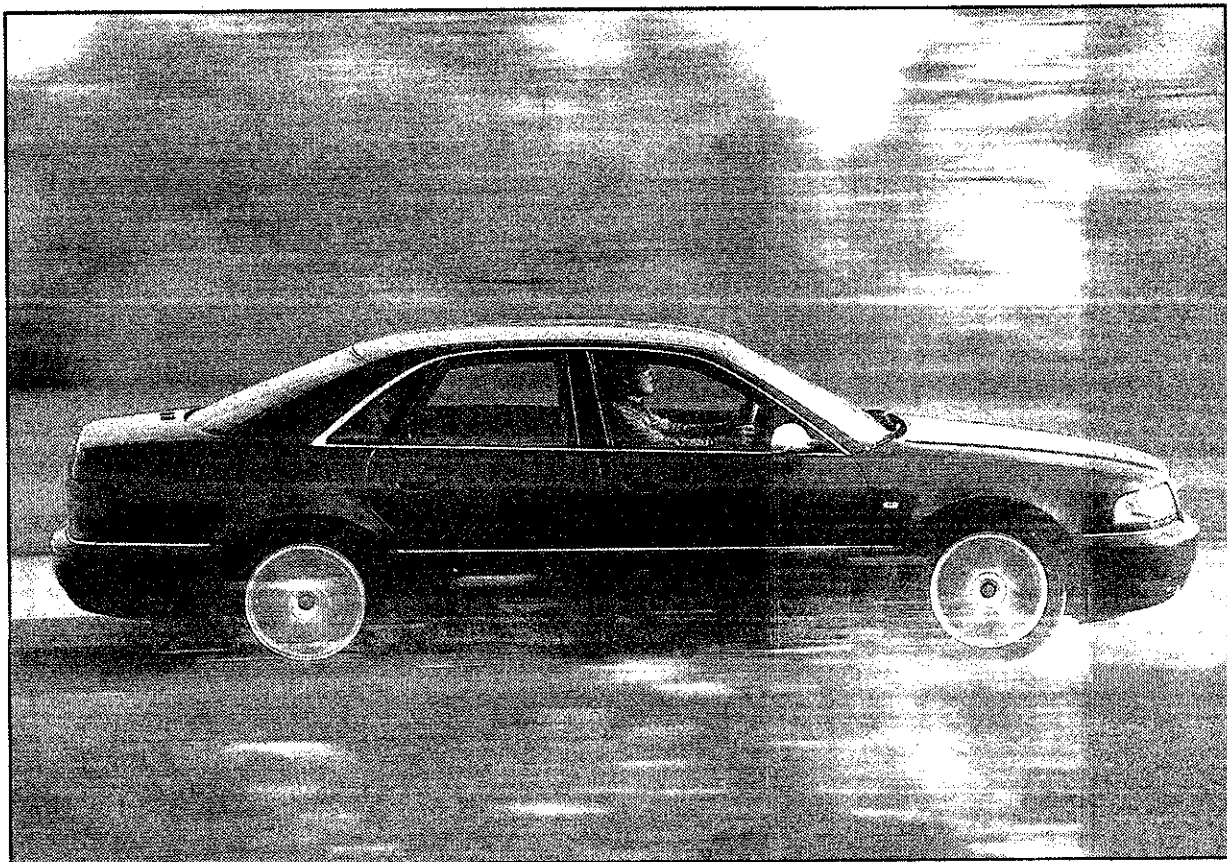
Classy chassis: The Audi S8 is a high-performance luxury car with an all-aluminum "Audi Space Frame" and a five-valve, 360-horse, 4.2-liter V8 mill.
