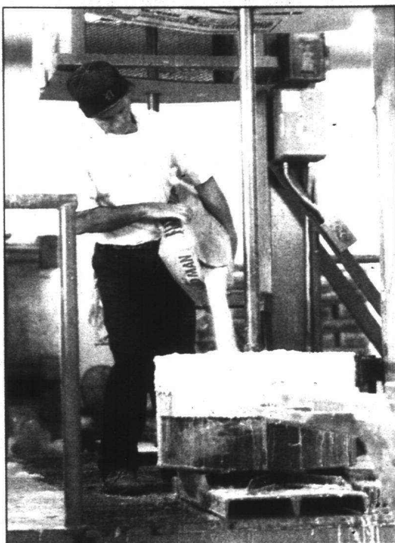
Mixing product: Above, Vitorio Muglia of Metro Cast adds sand to resin to produce a polymer concrete mixture.
