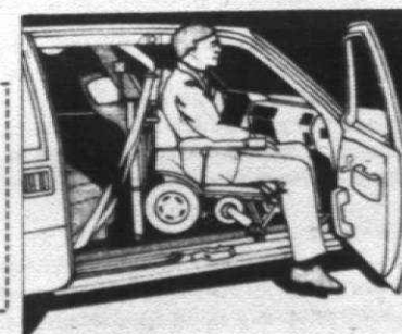
3. The wheels retract and CARCHAIR swings into car.
