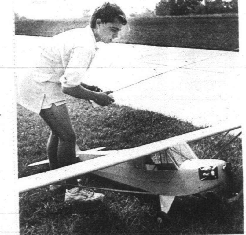
After the craft lands, Bert Brian Jr. will shut off the engine. This plane is powered by a quiet, four-stroke engine instead of the more common, but noisier, two-stroke.
