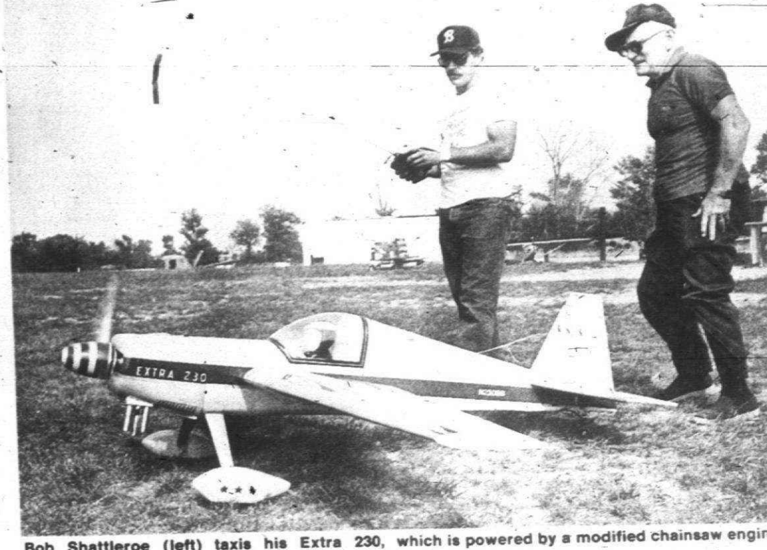
Bob Shattlerow (left) taxis his Extra 230, which is powered by a modified chainsaw engine. It can fly at speeds up to 100 mph.
