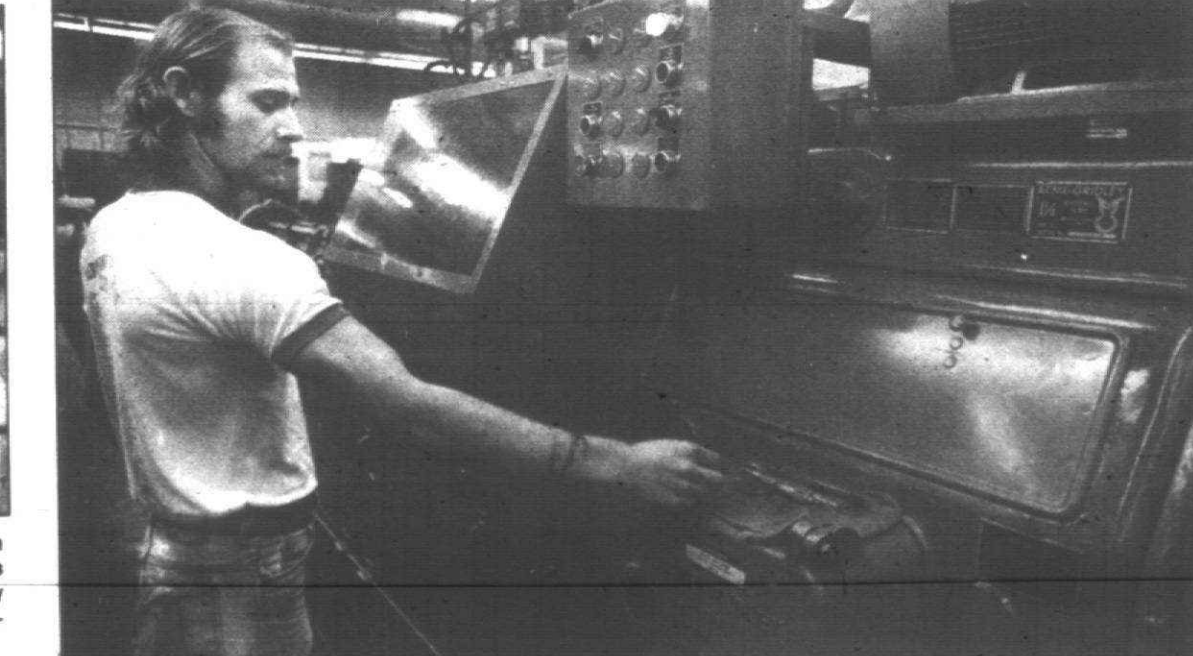
David Hoskins of Canton operates a milling machine that turns out tiny parts from long bars of aircraft-grade steel.
